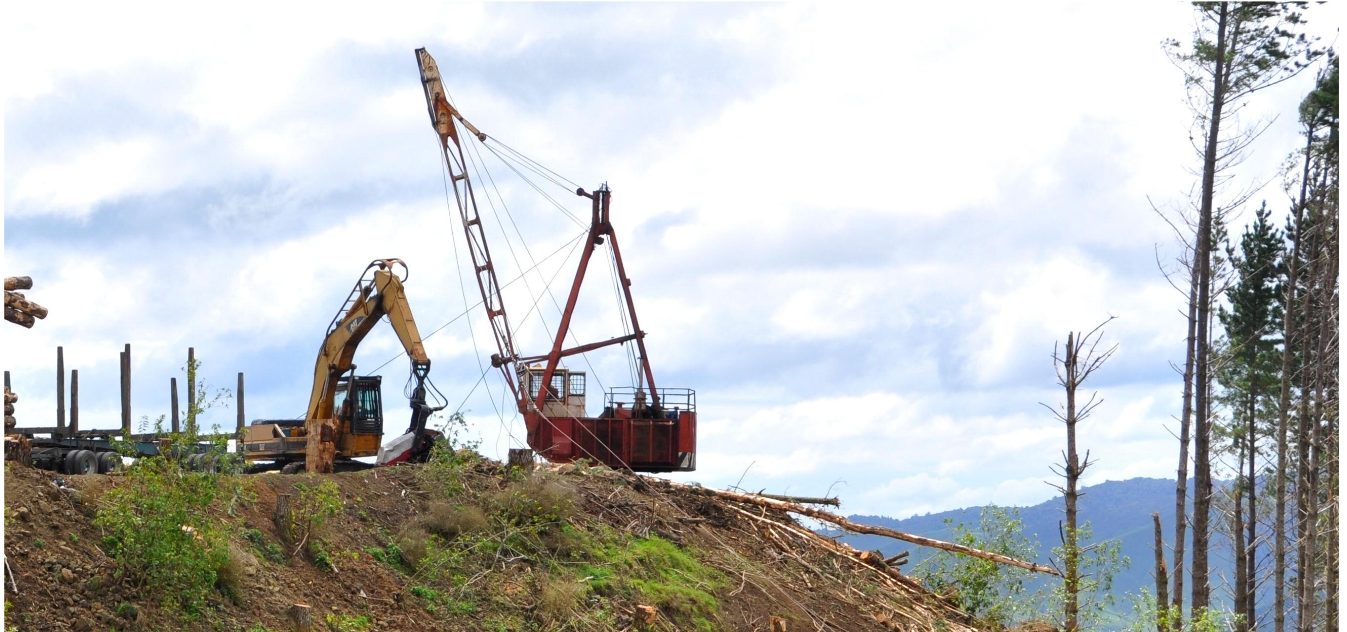
Photo: Harvesting in Mangakahia – logs are harvested and pulled up via cable and then stored at the landing site
